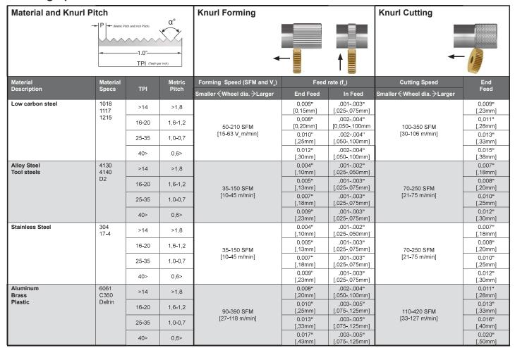
Note: When knurling, start with low Cutting speed, to evaluate the wheel performance, (to avoid the premature life of the wheel) increase until optimum cutting speed and feed is achieved
